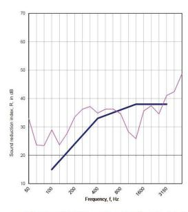
$D_{n,e,w}$  = 34 dB  $D_{n,e,w}$ +C = 32 dB  $D_{n,e,w}$ +C<sub>tr</sub> = 31 dB
