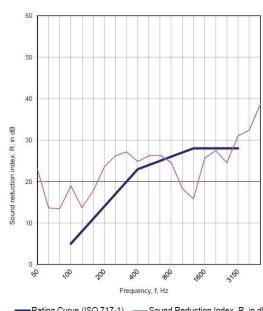
Rating Curve (ISO 717-1) — Sound Reduction Index, R, in dB
