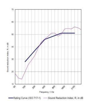
$R_w$  = 47 dB  $R_w$ +C = 45 dB  $R_w$ +C<sub>tr</sub> = 38 dB
