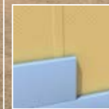
WT protection sheet / felt and thermal insulation boards
